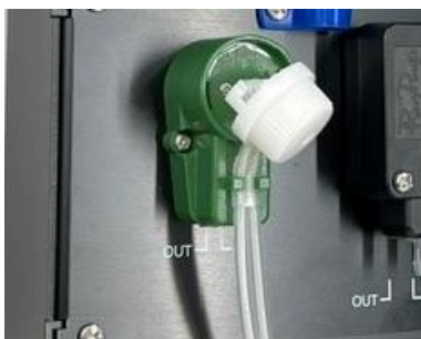
The head can be removed by turning it slightly counterclockwise.
